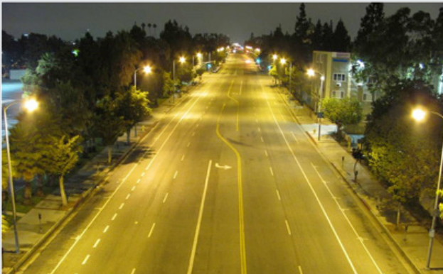
Figure 3. Visible non-uniformities characterize illumination from HPS and other bulb-based products.
